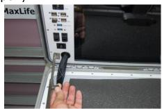
NOTE: Be sure to remove any USB plug-ins from the HUB prior to closing the lid. Shut off the keyboard and place packing foam inside case to protect the PC and prevent peripheral devices from sliding around in the case while in transport.
